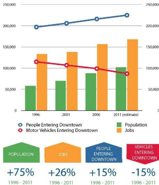
Figure 1: Population and Job Growth vs. Vehicle & Person Trips Downtown Vancouver, 1996-2011 (Peak Periods: 7-9 am, 11am-1pm, 3-6 pm)
